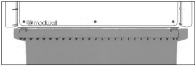
Step 7. !NB! Be sure to tuck the waterproofing sheet into the water tank, this is to prevent water dripping out behind the tank. Cut waterproofing sheet to size where needed.
