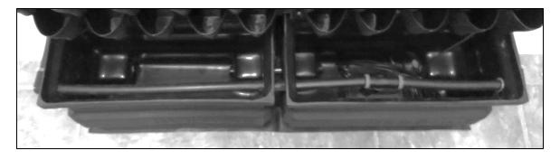
Step 35. Connect the final piece of pipe to the pump
