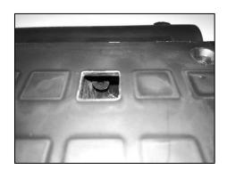
Use a piece of wire and clear the blockage in the nozzle, through the hole in the panel. Below is a picture of what the nozzle looks like, and how deep the wire needs to go to unclog the nozzle
