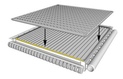
Recommended Tip: Use silicone around the bottom edge before fastening the grid onto the panel, as seen along the yellow line above. This is to ensure water stays inside the panels, but isn't essential
