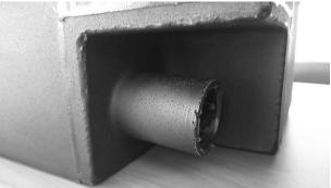
Step 2. Place the rubber hose over the openings, and fasten clamps tightly
